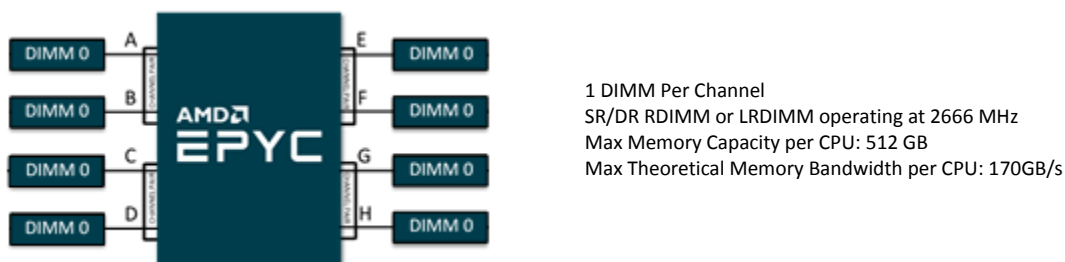
Figure 4. Sample Configuration for Memory Bandwidth Sensitive Workloads
