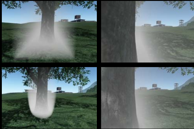
Rendering of fog volumes: Box (top left/right), Ellipsoid (bottom left/right)
