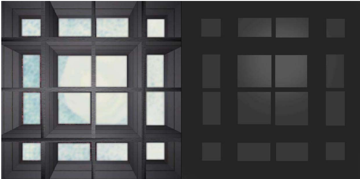
Figure 4: Top face of HDR cubic environment map (left) RGB Channels (right) Alpha Channel.
