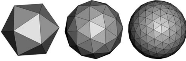
Figure 4: Viewpoint generation. A series of progressively denser viewpoint sets can be produced by subdivision of an icosahedron. From left to right, sets of 12, 42, and 162 viewpoints.
