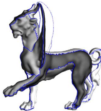
Figure 3: The Feline mesh partitioned into 32 planar patches. Notice how patches tend to follow the natural creases of the mesh. This is due to our normal-based clustering metric.
